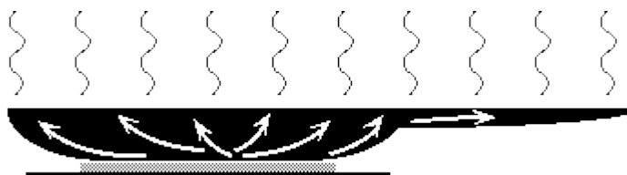
Figure 5. Heat conducted through the pan to handle
