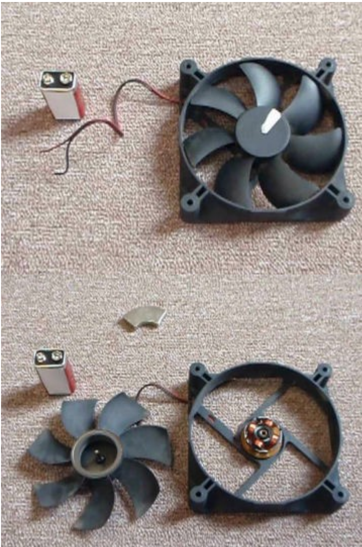
A computer fan can be used to build a small prototype of the magnet motor. You can see the motor before disassembly (left) and after disassembly (right).
