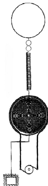
Fig. 4 Oscillating electrostatically charged dome.
